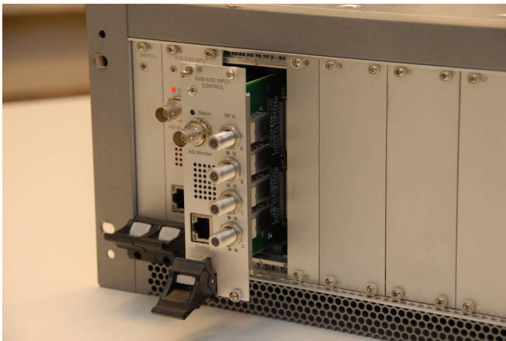
Figure 14.1 - A Module with its Ejector released
