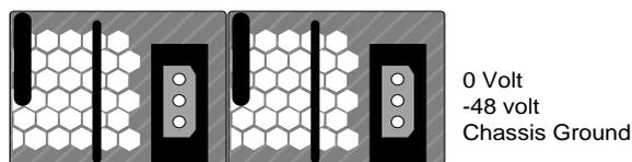
Figure 2.12 Power Input Connector for 1RU Chassis, product models XC5100 with DC power
