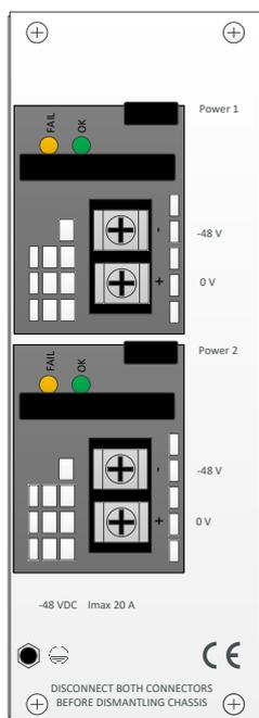
Figure 2.10- Power input for 4RU chassis with 800W DC power supplies
