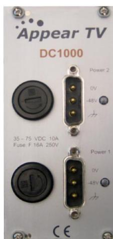
Figure 2.8- Front plate of dual 48V Power Supply in a DC1000
