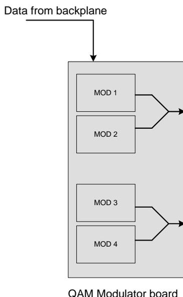
The QAM modulator consists of four modulator chips, each carrying up to 4 carriers. The frequency is set only for the first carrier of each modulator. The remaining three carriers per modulator follow regular spacing.
