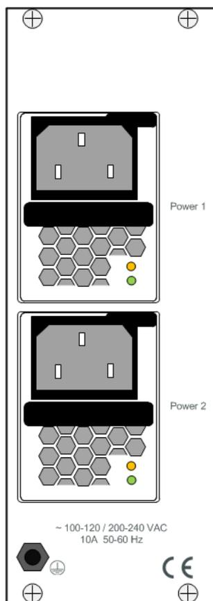
Figure 2.7- Power input for 4RU chassis with 800W AC power supplies
